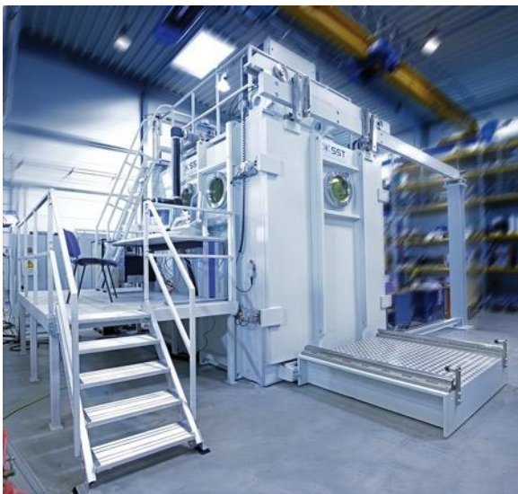
Caption: Modern universal electron beam machine from Steigerwald Strahltechnik
